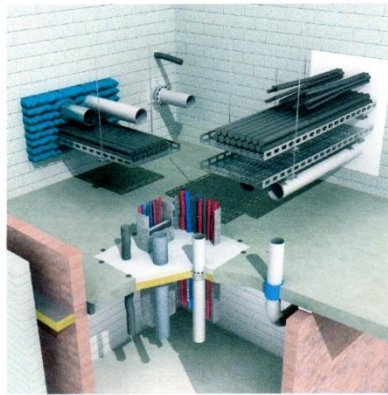
Figure 1 – typical applications for fire-stopping systems
