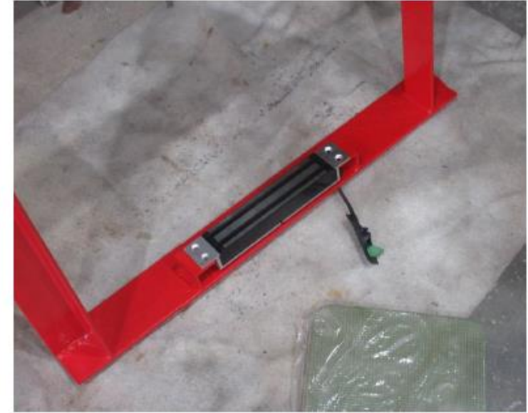
Photo 5. Installation of mag lock 600M onto Main frame.
