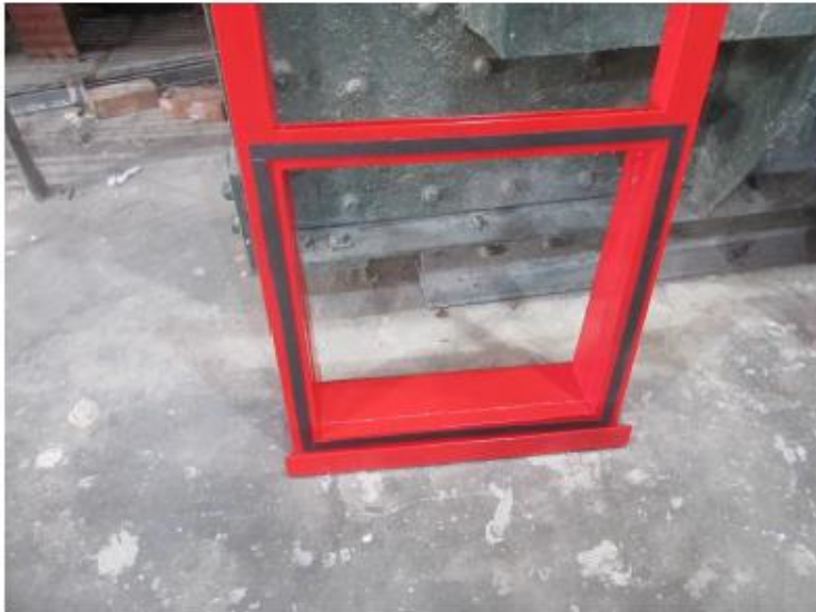
Photo 4. Thermaflex Intumescent strip applied to the underside of Main frame.
